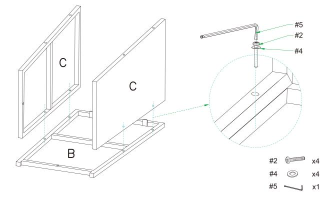
**Step 2.** Attach bottom panel (part D) to side panels (part C) and front panel (part B) using long bolts (part #2), washers (part #4) and allen key (part #5).
