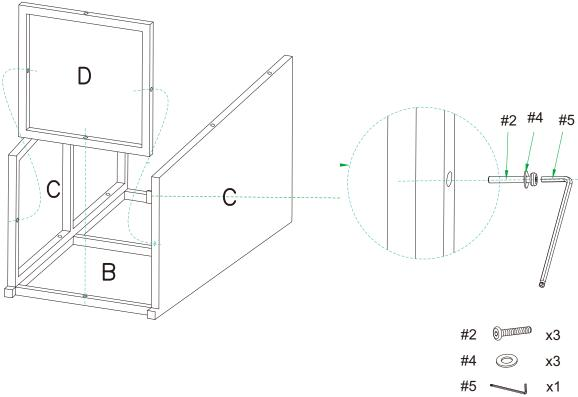
**Step 3.** Attach back panel (part A) to side panels (part C) and bottom panel (D) using long bolts (part #2), washers (part #4) and allen key (part #5).
